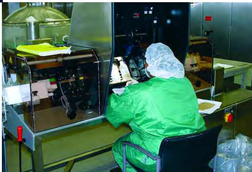
bottle is automatically spun around to make sure every millimeter of its surface is examined. To ensure acuity and attention, the inspector—another green-clad body sitting with his or her head resting about a foot behind the magnified viewing glass—is rotated out every 30 minutes. ➤
